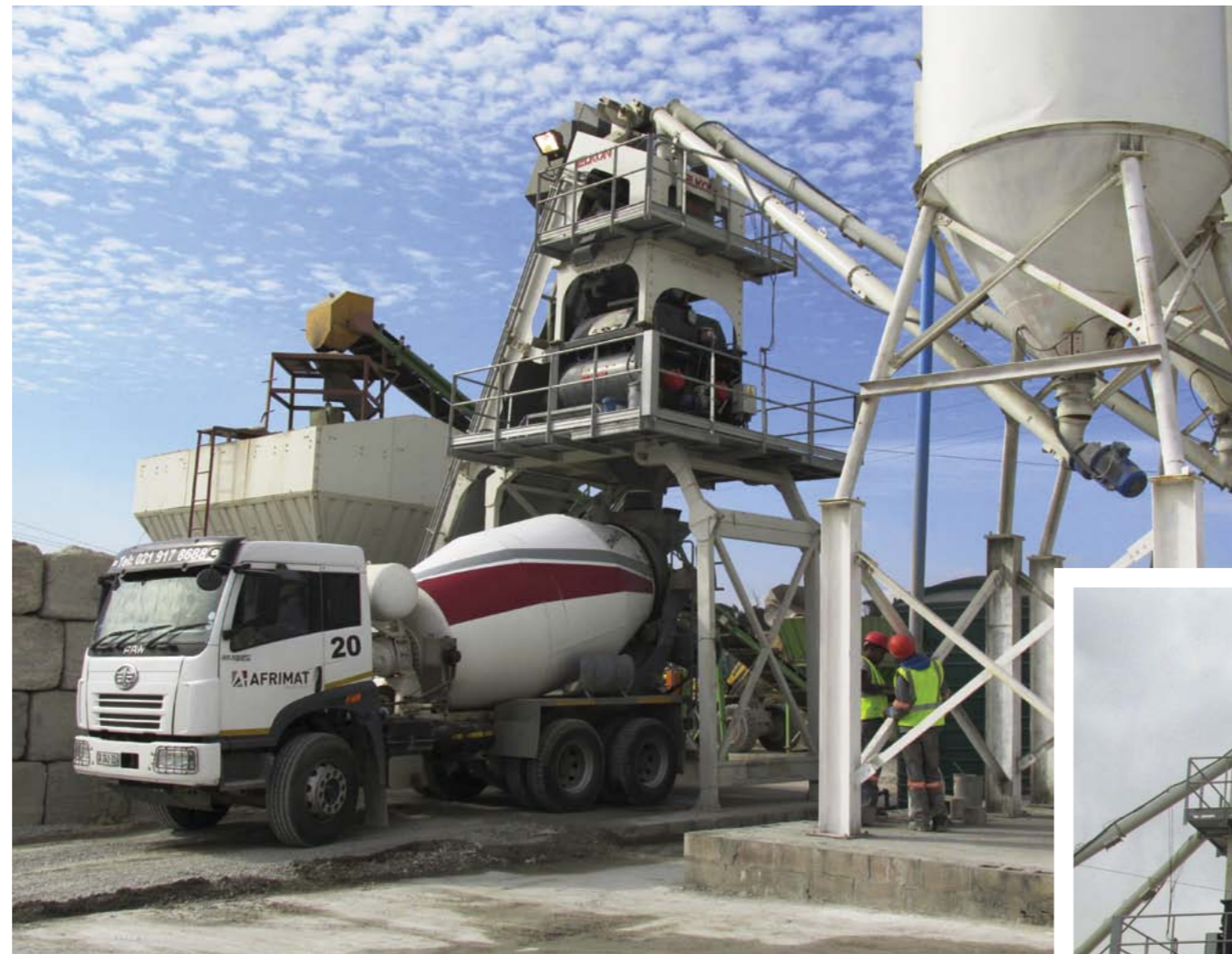
The Elkon Quick Master 60 is Afrimat Readymix's second Wet Batch plant.
