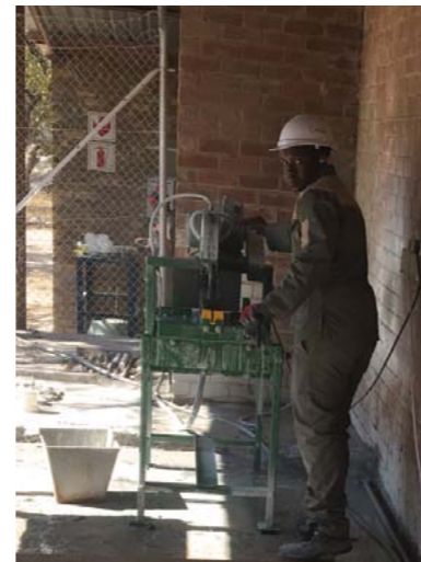
Above left: Detail of core sections placed into core trays Above Right: Cores being cut in half along their length Left: Core trays packed for sampling in the core yard Below: Completed trays labelled for transport
