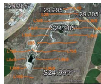
Above left: Aerial photograph of southern mine area with superimposed X-Y Gridlines at 500m intervals Above right: Satellite image with superimposed orange lines to map rock resistivity
