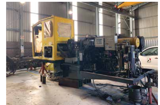
The HDR7 being rebuilt
