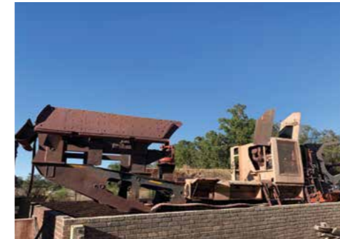
LT3054 with crusher, feeder and discharge conveyor removed
