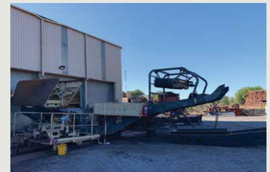
LT105-2 with crusher removed. This was rebuilt with parts from an old LT105-3
