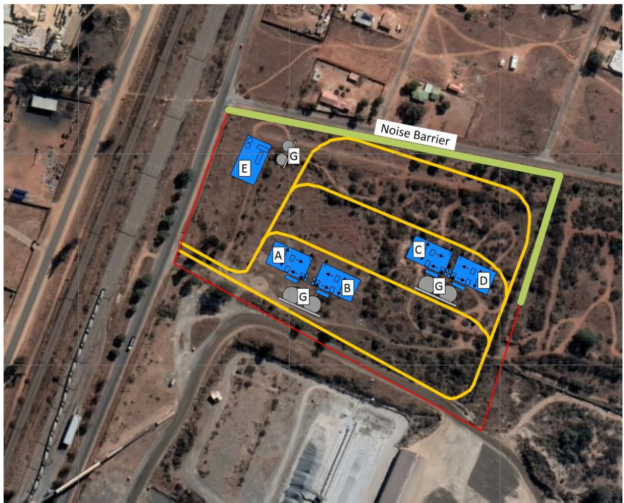
Figure 7-1 Position and alignment of a noise barrier for acoustic screening of reverse alarm noise
