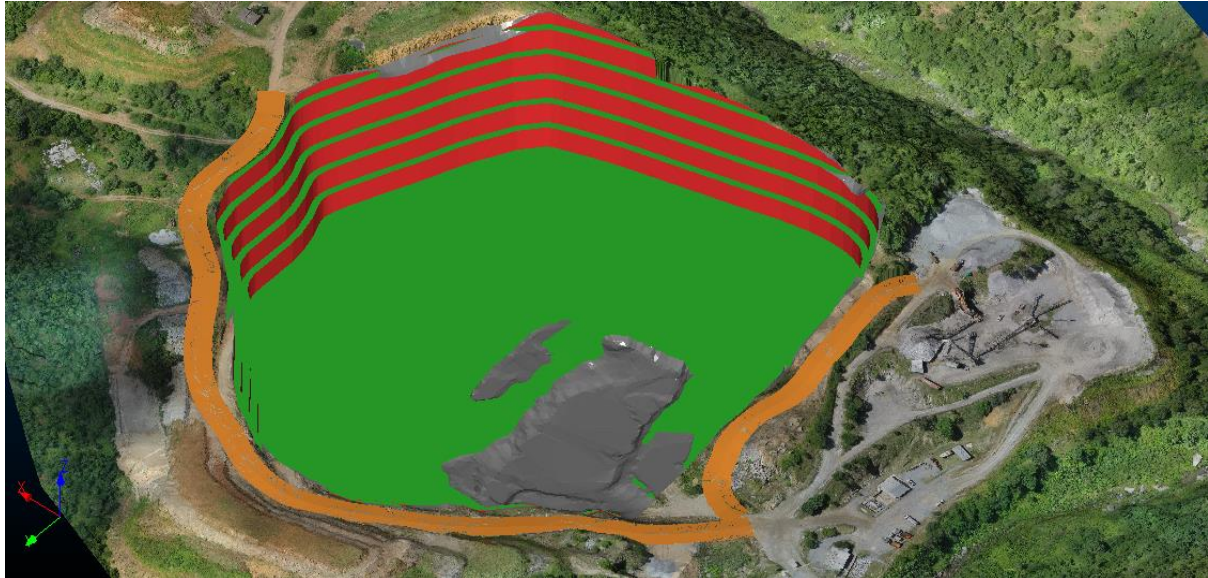
Figure 7: Pit design with surface roads
