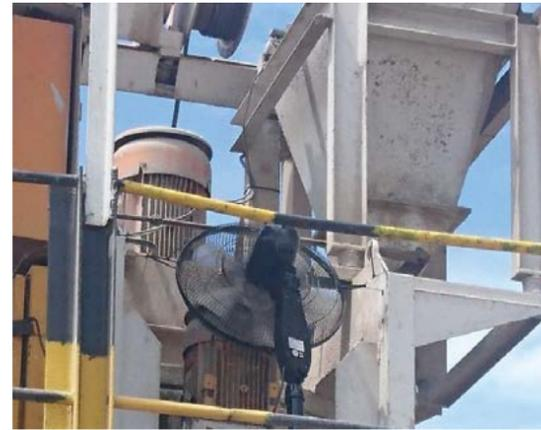
Office fan used to cool off the overheating electric motor
