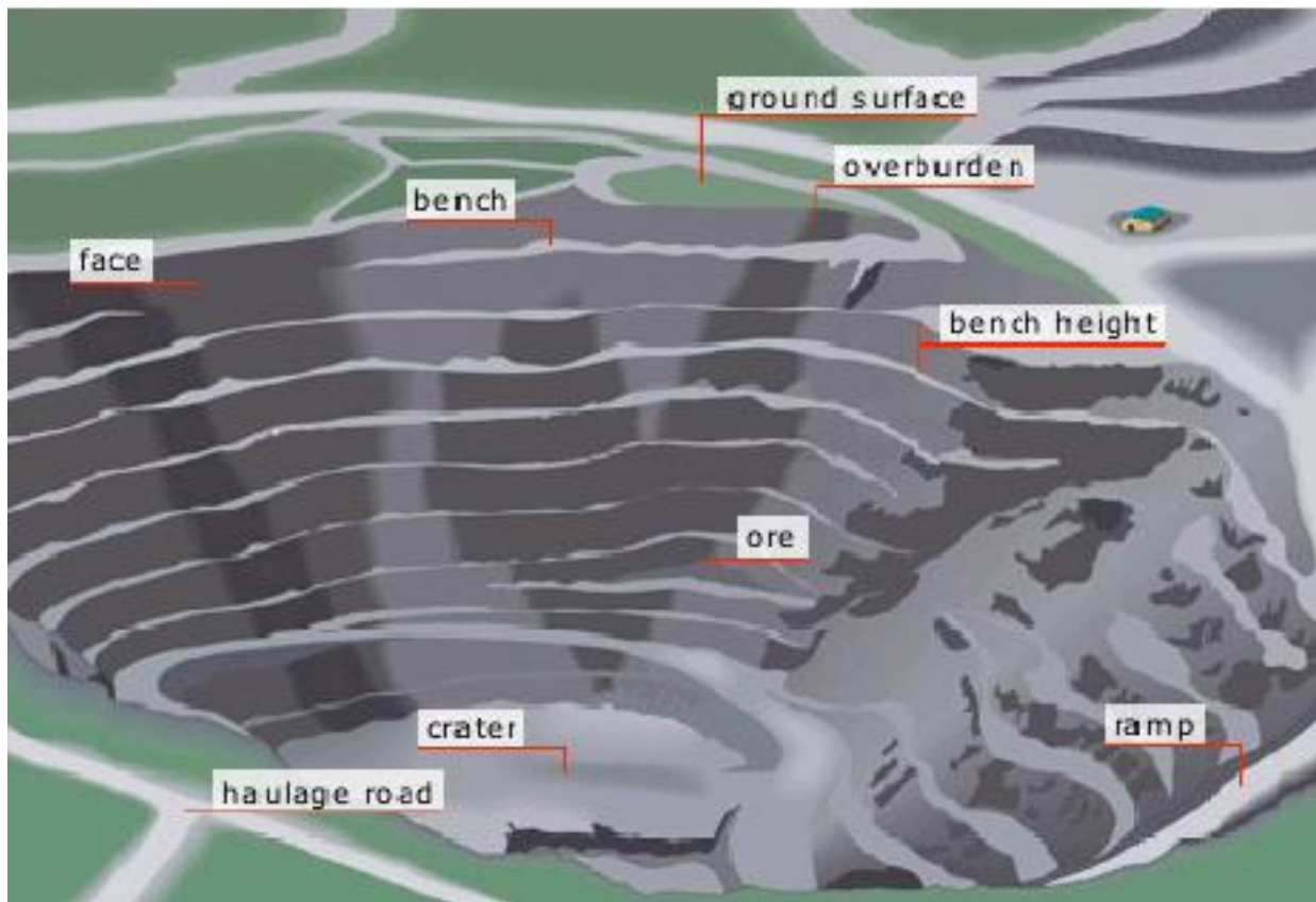
Figure 7: Schematic illustration of an open pit mine
